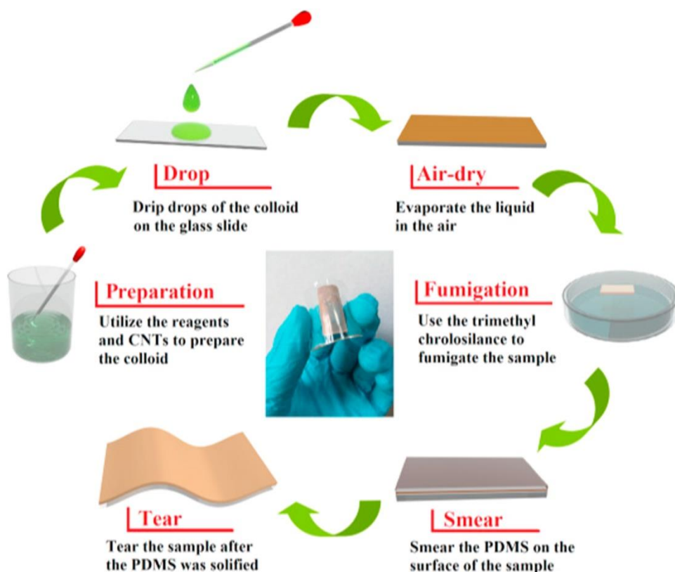
Figure 4. 15: The strain sensor fabrication process over PDMS substrate with CNTs modified of Ag NPs. The final product is illustrated at the center of the figure. Copyright permission from [306].
