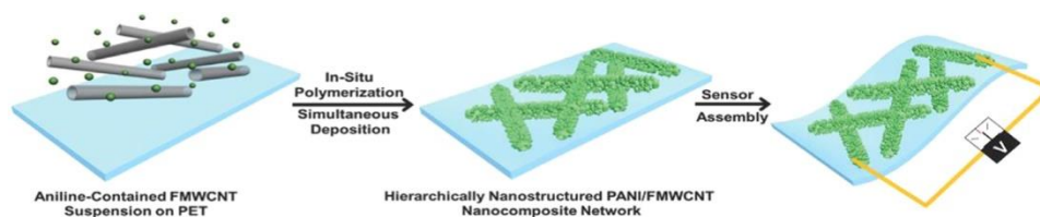
Figure 4. 18: Schematic graphical representation of the development of flexible sensor based on nanocomposite PANI/F-MWCNT on flexible polyethylene terephthalate (PET) substrate.
